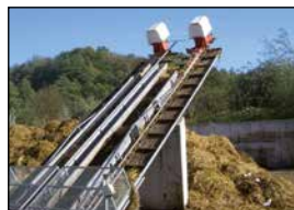
▲ Rope-/chain dunging for horse stables
