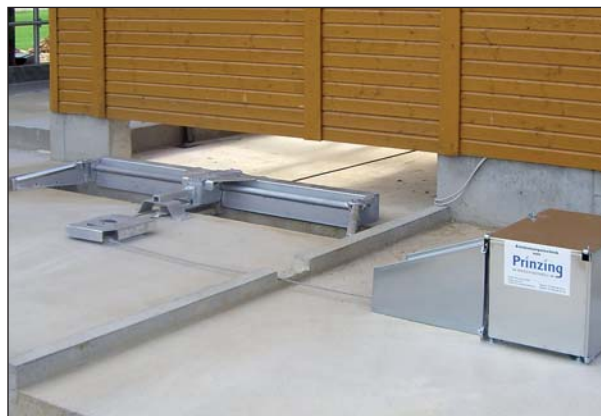
▲ Assembling drive winch EW4, guide pulley and flap scraper PKSF
