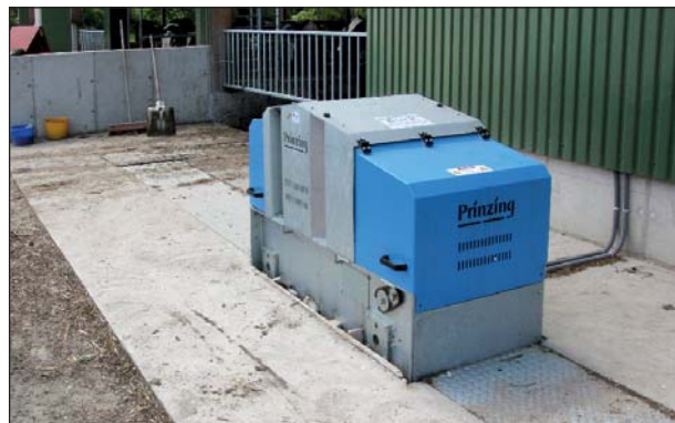
▲ Double drive winch DW7 with rope guidance in a covered floor channel
