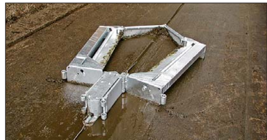
▲ Flap scraper, base frame pivotable
